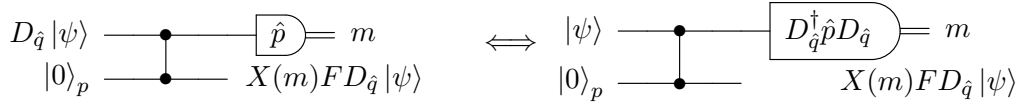
Figure III.3: Implementation in an MBQC fashion of D_{\hat{q}} , an arbitrary unitary evolution diagonal in \hat{q} . |0\rangle_p is an infinitely momentum squeezed state. Left : the gate is applied directly on the quantum state |\psi\rangle before teleporting it. Right : the gate is applied by measuring the state |\psi\rangle in a different basis.
