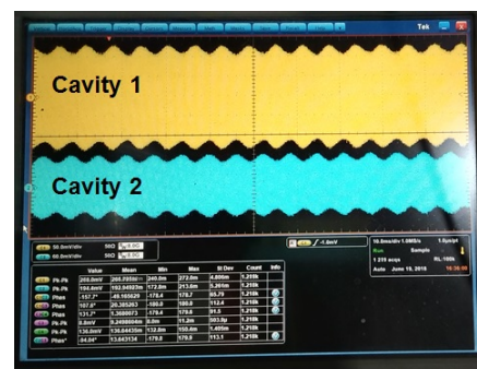
Figure 2: Experimental results: Pick-up signals of 2 cavities in vector sum control after several seconds of operation. Mechanical resonance frequency is roughly 160 Hz and the RF bandwidth is roughly 300 Hz.
