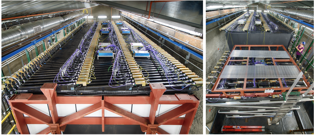
Figure 3.9: Photographs of the near detector, composed of the active region and the muon catcher. Left: the front of the detector. Right: the downstream end of the detector is the muon catcher. Taken From [59].
