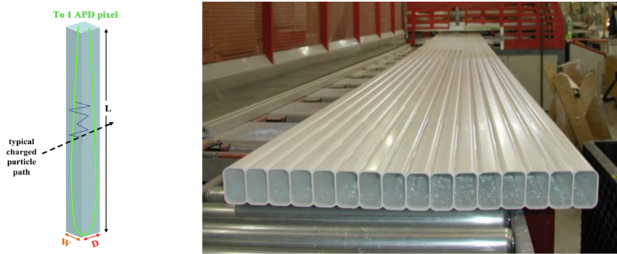
Figure 3.7: Left: diagram of a cell. Right: photograph of one PVC extrusion. Taken from [57].
