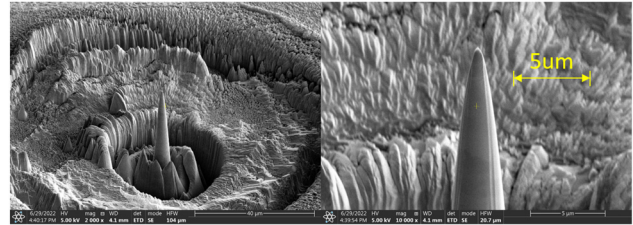
Figure 2: Nanotip fabricated by annular FIB.
