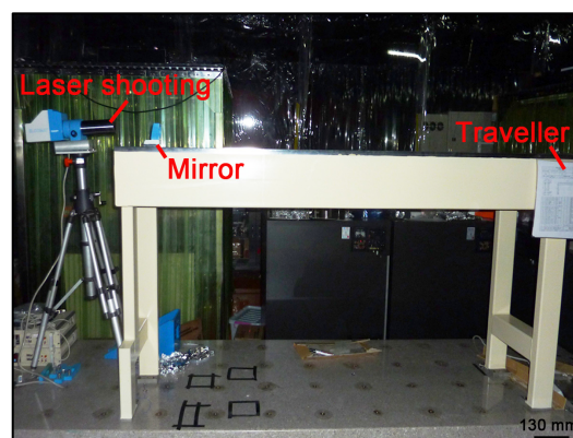
Figure 2: Measurement and erection of laser alignment tool.
