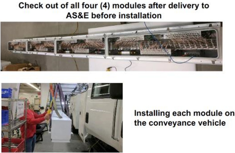
Fig. 7. Installation of the four HiRIS detector modules onto the VACIS truck.
