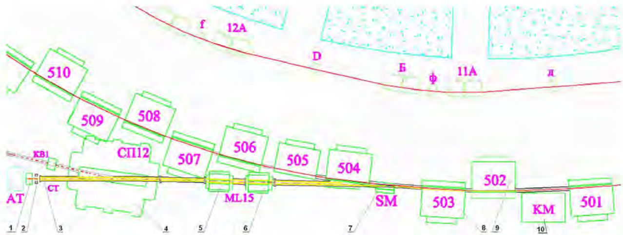
Fig. 9: The facility schematic and the fast extraction units: 1. Table to place the samples to be irradiated. 2. Current transformer. 3. Outlet flange of vacuumized proton guide. 4. Bending magnet. 5, 6. Doublet of quadrupole lenses. 7. Septum magnet. 8, 9. Magnetic units of accelerating ring. 10. Kicker-magnet.
