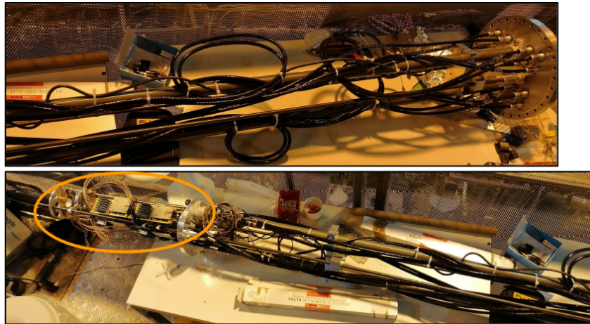
Figure B.5: On the top, picture of the upper part of the nearly 2.5 m long WISArD tower, which is vertically inserted inside the magnet section from the opening at the top of the cryostat system. At the bottom, a picture of the lower part of the tower, with an orange ellipse showing the zone in which the detection set-up, comprehensive of all the detectors and their respective preamplifiers, is located.
