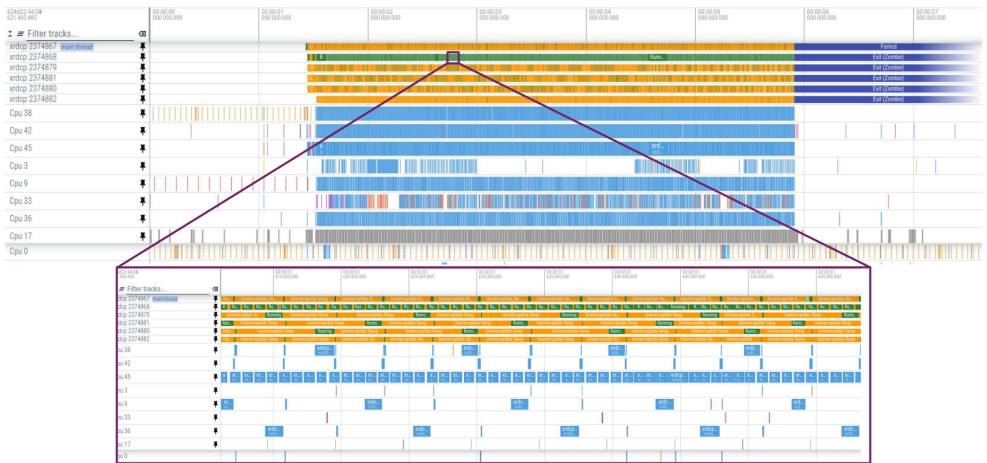
Figure 10: XRootD client in 100GbE networking environment. One thread is CPU bound, while other threads remain mostly idle.
