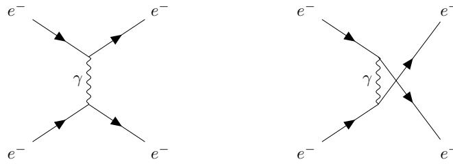
Figure 2.2: Feynman diagrams for electron–electron QED interactions.
