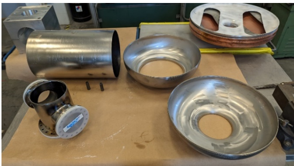
Figure 7: Niobium subcomponents of the 591 MHz cavity.
