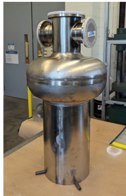
Figure 8: Subcomponents stacked into the 591 MHz cavity (not welded yet).
