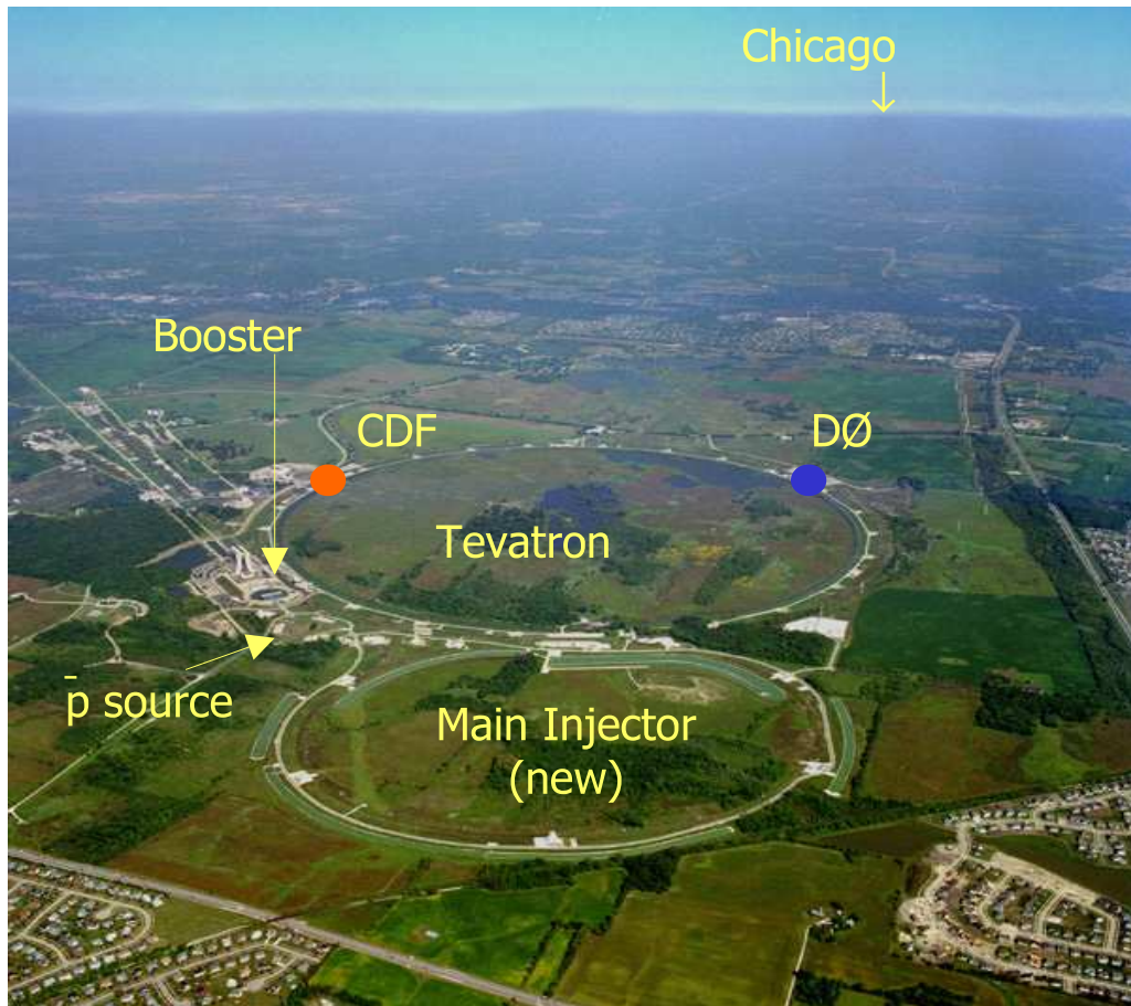
Figure 3.1: Aerial view of the TeVatron accelerator complex at Fermilab near Chicago. The foreground shows the Main Injector while the main TeVatron accelerator with its two experiments CDF and DØ is the ring of 6 km circumference, visible in the background.
