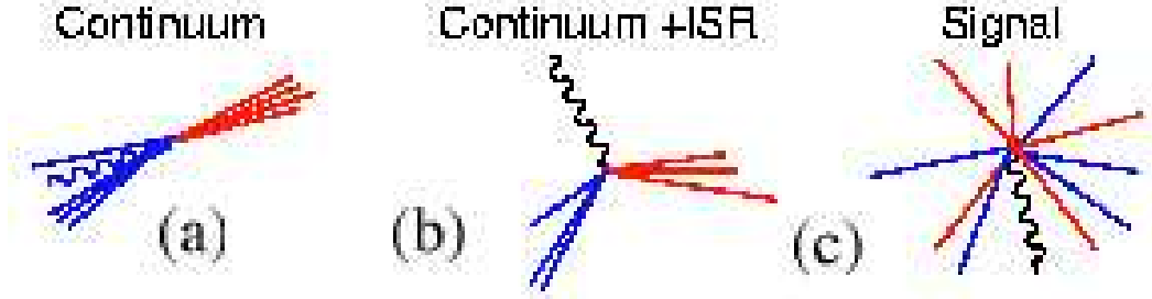
Figure 5.3: Event shape for (a) \pi^0/\eta continuum background (jet-like), (b) continuum background (ISR) and (c) signal decay (spherical) in the c.m. frame.
