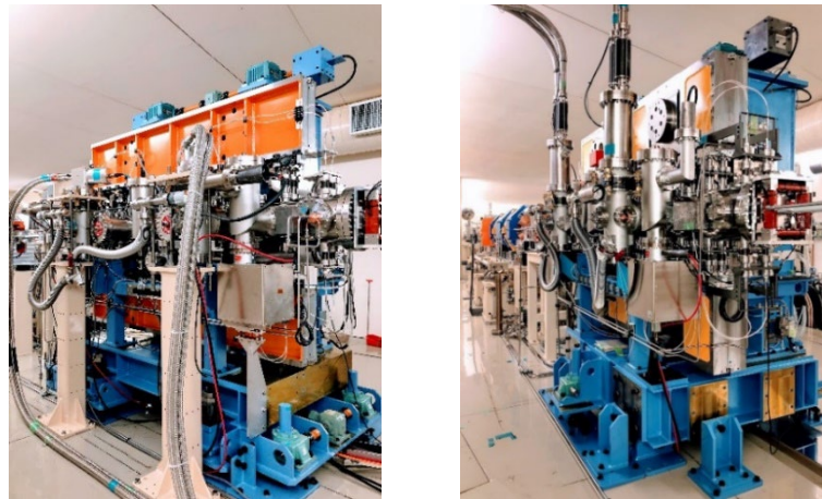
Figure 2: (left) CU15 installed for the high-resolution powder diffraction TPS 19A beamline; (right) CUT18 installed for the advanced microcrystal chemical crystallography TPS 15A beamline.
