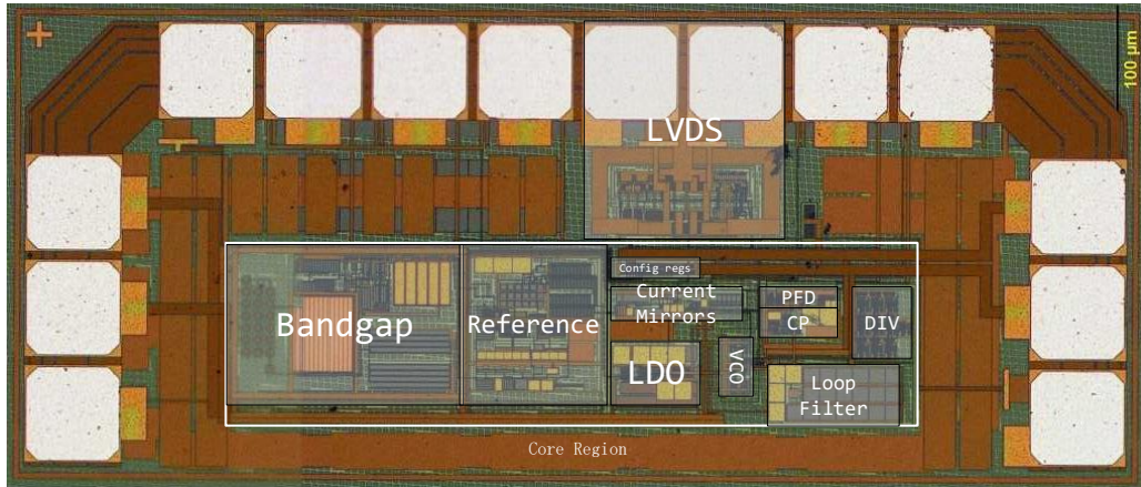
Figure 5.12 Layout of PLL-0.
