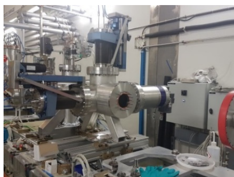
Figure 2: EM installed on injection channel of linac accelerator. Double-unit configuration used for 2+2 D scan installed in same focusing plane. The actuators and mechanical structures in blue, bellows and flanges with feed-throughs.
