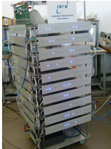
Figure 4. The compact cosmic ray telescope developed at LNGS. A multi-track is visualized by using LED matrices in double view.
