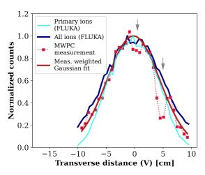
Figure 2: Comparison between the FLUKA simulated beam sizes for primary ions only (cyan), all ions (navy), and measurement data from the MWPC (red squares). A weighted Gaussian fit of the data takes into account instruments and support frames in the "view" of the MWPC (arrows).
