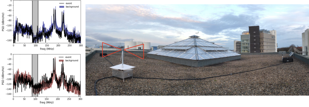
Figure 3: Right: Prototype array station located on the roof of the Vrije Universiteit Brussel. The antenna is highlighted in the center, with scintillators housed in black boxes on either side. The roof prototype uses CODALEMA butterfly antennas, while the field setup will use SKALA antennas. Left: Power spectra for a sample event. The average background is shown as the shaded colored background. The region of a FM bandpass filter is shown in gray.
