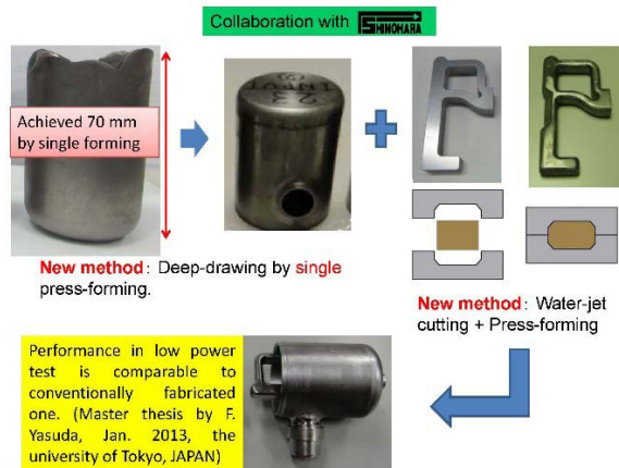
Figure 6: The new fabrication-methods for the HOM coupler for KEK01 cavity.
