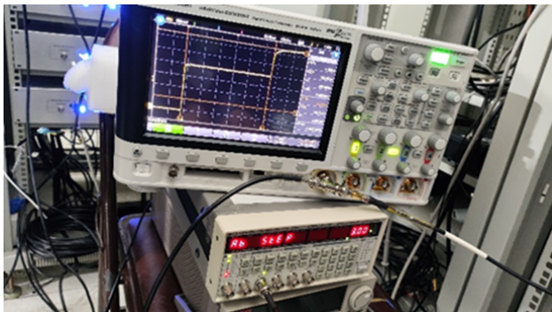
Figure 3: Measure cable delay using an oscilloscope with a function generator.
