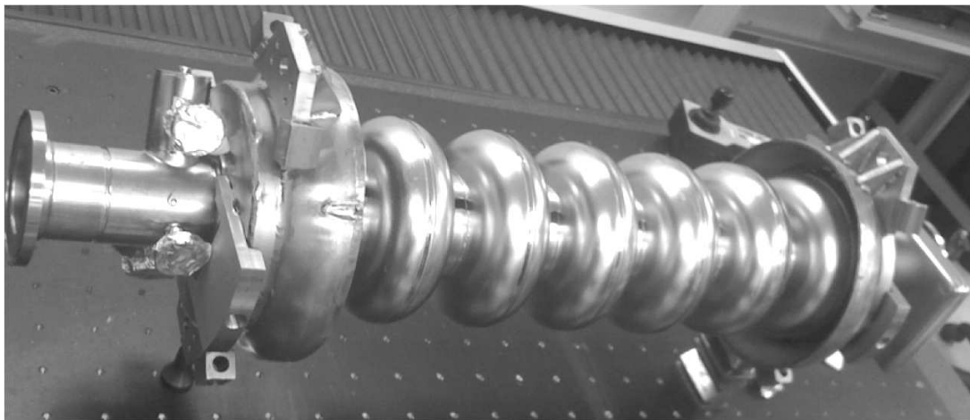
Figure 10. Image of a new high gradient and low loss cavity used to increase the CEBAF base energy to 6 GeV as well as prepare for the 12 GeV upgrade.
