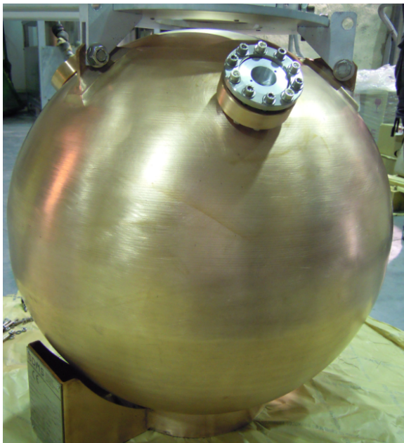
Figure 1. Picture of SEDINE, a 60-cm diameter prototype SPC installed at the LSM in Modane.
