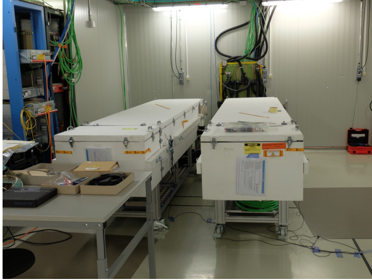
Figure C.1. Photo of the pixel lab at the CMS experimental site, showing two of the FPIX cold boxes, with the system of cooling pipes in the back bringing water-glycol and C_6F_{14} to cool the interior of the boxes, and the power supply and DAQ crates (blue) to the left for reading out one half-cylinder at a time.
