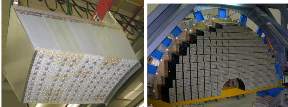
Figure 2.13. (Left) Module from the ECAL barrel. (Right) Supercrystals mounted on an ECAL endcap Dee. [24]
