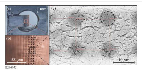
**Figure 3.** Microchannel array targets used in the TPW campaign: (a) mounting of target on carbon fiber slide; (b) zoom in on front surface of microchannel array; (c) SEM of  $6 \mu m$ -ID channels (black dashed, example) filled with low-density CH foam. The CH foam produces the submicron structure visible on the surface of the target.
