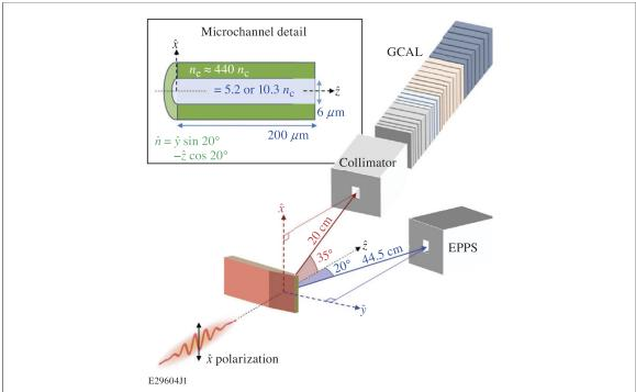
**Figure 4.** Schematic of the experimental geometry. EPPS is positioned  $20^{\circ}$  off the laser/microchannel axis in the perpendicular direction  $(\hat{y})$ ; GCAL is positioned  $35^{\circ}$  off-axis in the polarization direction  $(\hat{x})$ . (Inset) Detail on geometry of microchannels in array target.
