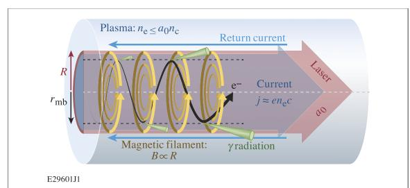
**Figure 1.** Schematic diagram of the relativistically transparent magnetic filament phenomenon. An intense laser (red) drives a relativistic current (blue) in a relativistically transparent plasma. The azimuthal magnetic field (orange) traps electrons (black) either within the laser radius R or a magnetic boundary  $r_{\rm mb}$  (see text). Electrons are directly accelerated by the laser fields and radiate high-energy photons (green).
