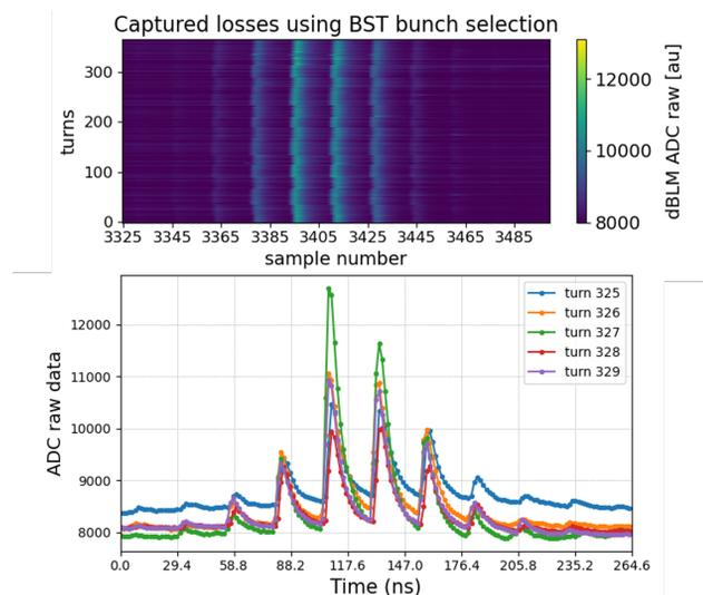
Figure 5: Capture data on selected bunches. Top: reconstruction with 365 turns. Bottom: Zoom on turns 325-329.
