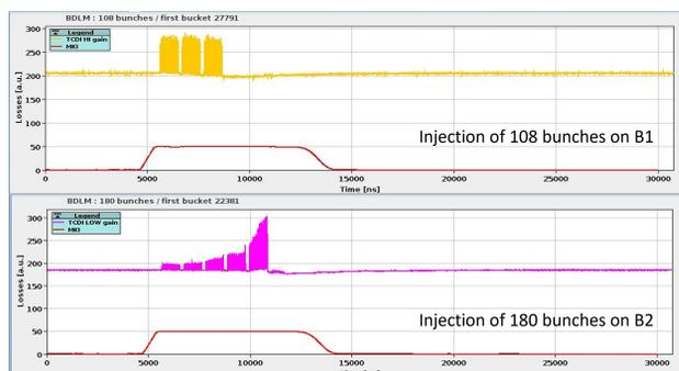
Figure 6: IQC screenshots showing injection data from the dBLM monitors in the LHC injection lines.
