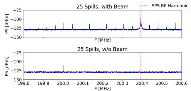
Figure 7: FFT data around the SPS RF nominal frequency as measured by diamond BLM detectors on the TT20 slow extraction line.
