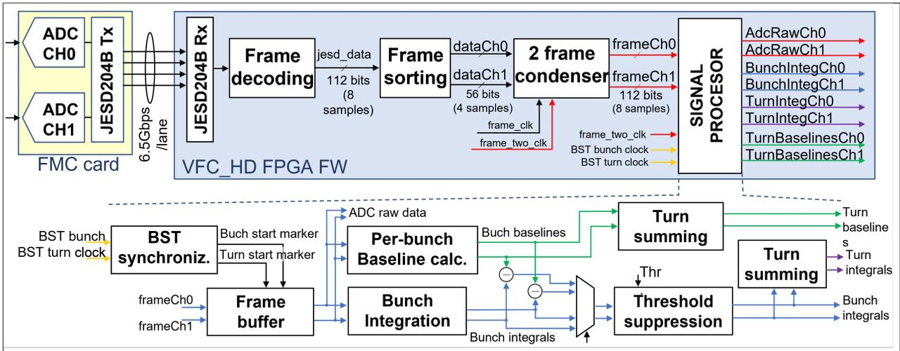
Figure 4: Simplified functional block diagram of the LHC and SPS diamond BLM firmware.
