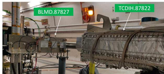
Figure 2: Photo of a dBLM detector installed at the end of the T18 LHC injection line.
