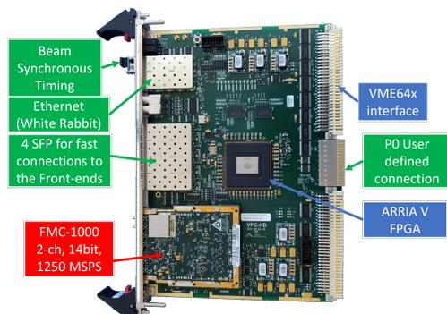
Figure 3: Photo of the VFC-HD card with a FMC-1000 card.
