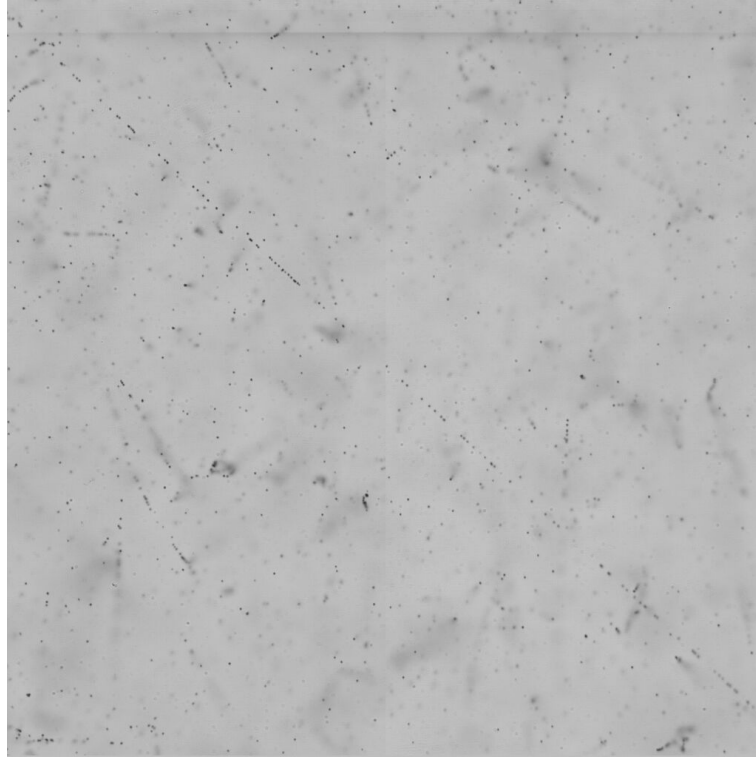
Figure 5.4: An image showing a typical emulsion view; a magnification of 50x is applied, the image sensor size is 1024 \times 1024 pixels and the field of view 244 \times 244 \mu\text{m}^2 .
