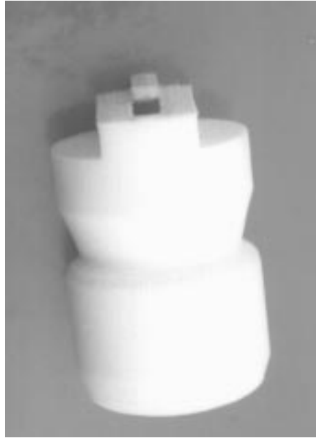
Figure 10: Photo of one of the “zips” used to insert the profiles in the 1997 and 1998 Modules 0.
