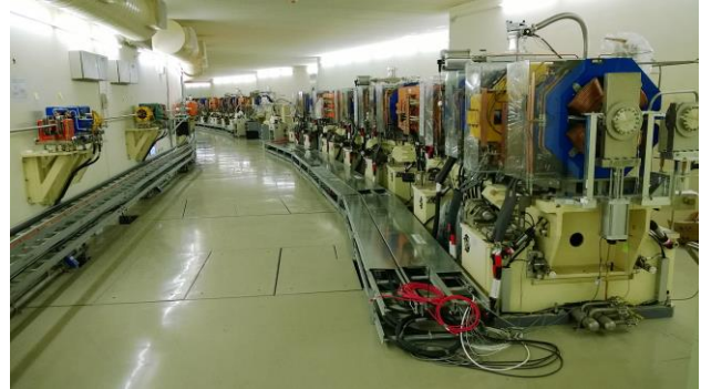
Figure 11: The whole ring girders installed at TPS tunnel
