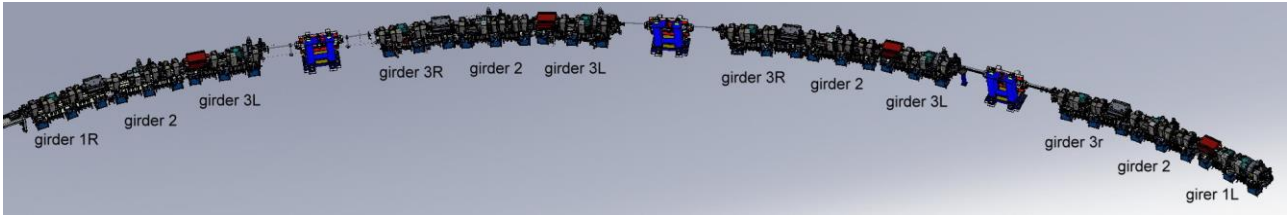
Figure 1: One superperiod girder configuration of the TPS storage Ring.
