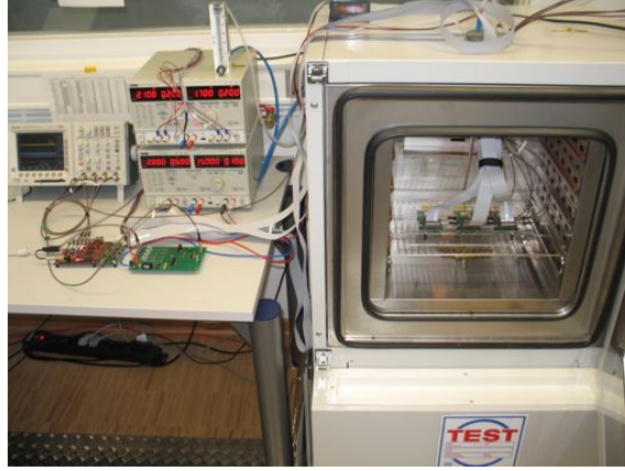
Figure 5.1: The USBpix test setup: the S3-Multi-IO-Board (DAQ computer not shown), LV power supplies (HV power supplies not shown), and the climate chamber.
