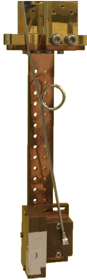
Figure 3.16: Device attached to the cold finger of a ^3\text{He} adsorption cryogenic refrigerator.
