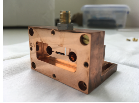
(b) 3D copper cavity represented by a loop-gap resonator.
