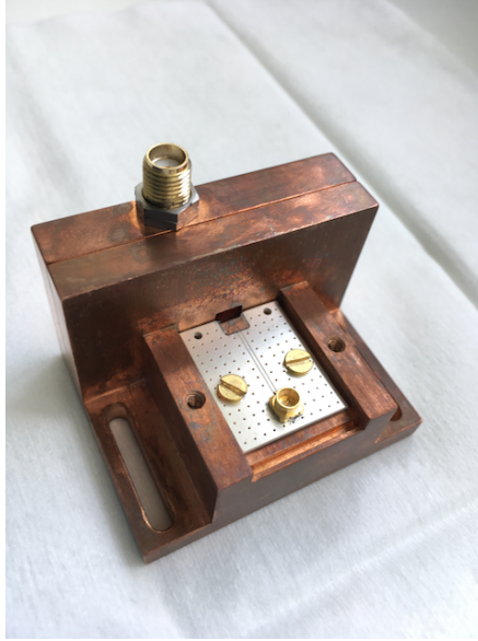
(a) Silicon chip with PCB mounted in a 3D copper cavity.
