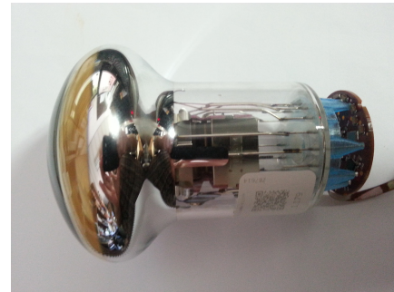
FIG. 78. A Hamamatsu R12199-02 7.7 cm PMT that is currently used in KM3Net and considered for IceCube-Gen2 modules. As this passed the Hyper-K PMT requirements, it is also a good candidate for a Hyper-K mPMT.
