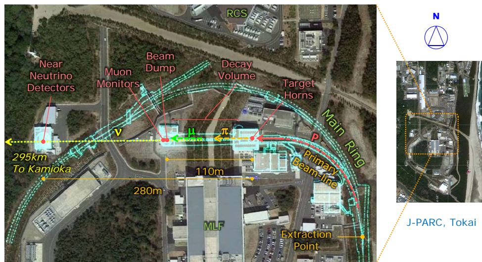
FIG. 8. The neutrino experimental facility (neutrino beamline) at J-PARC.
