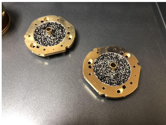
Figure 7.4: Tube electrodes of the Penning trap system with the activated charcoal for cryo-absorption. The activated charcoal is attached using a layer of the MCT 3715-2SE adhesive from MicroCoat Technologies.
