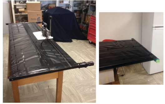
Figure 13. The OV top detector is shown. In the right panel a detail of one of the wavelength shifting plastic is shown.
