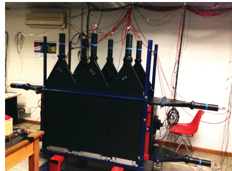
Figure 9. The prototype mounted and cabled at the INFN-Sezione di Catania. OV detectors are visible
