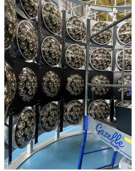
(b) All mPMT and some of the black sheet in place in the barrel.
