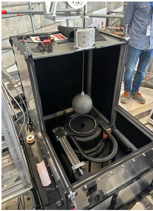
(a) Picture of the Ni-Cf calibration source about to be lowered into the tank by the CDS. Picture credit: WCTE collaboration.
