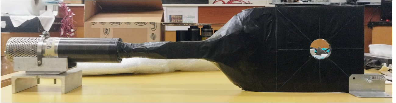
Figure 4.5: Picture of one of the hole counters composed of a hollow scintillator slab (right) coupled to a PMT (left). Picture by D. Divecha.
