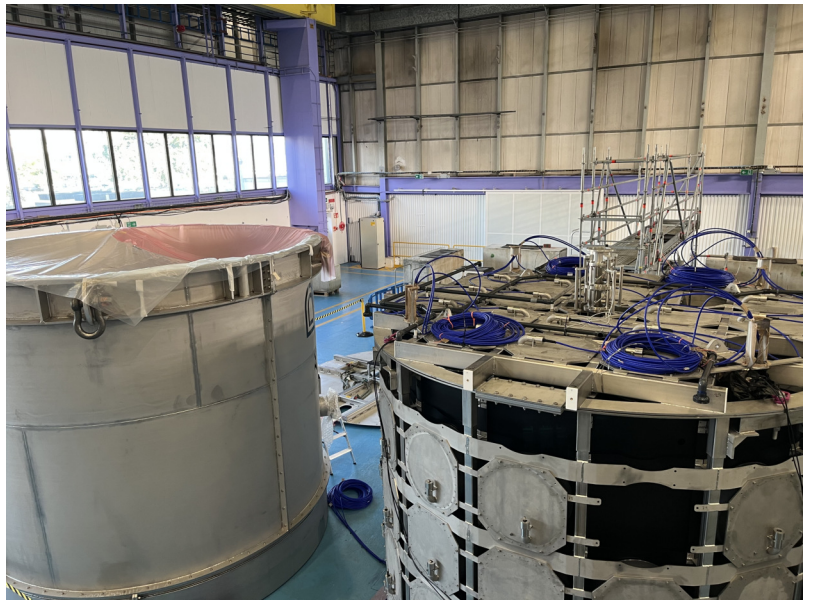
(d) The assembled inner structure (right) filled with mPMTs and fitted with the CDS arm next to the tank (left)
