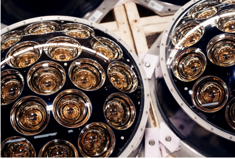
(a) Picture of WCTE mPMTs made with the in-situ (left) and ex-situ (right) gelling techniques.
