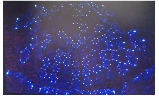
(c) Photogrammetry image with some of the mPMT slow LED used as light sources
