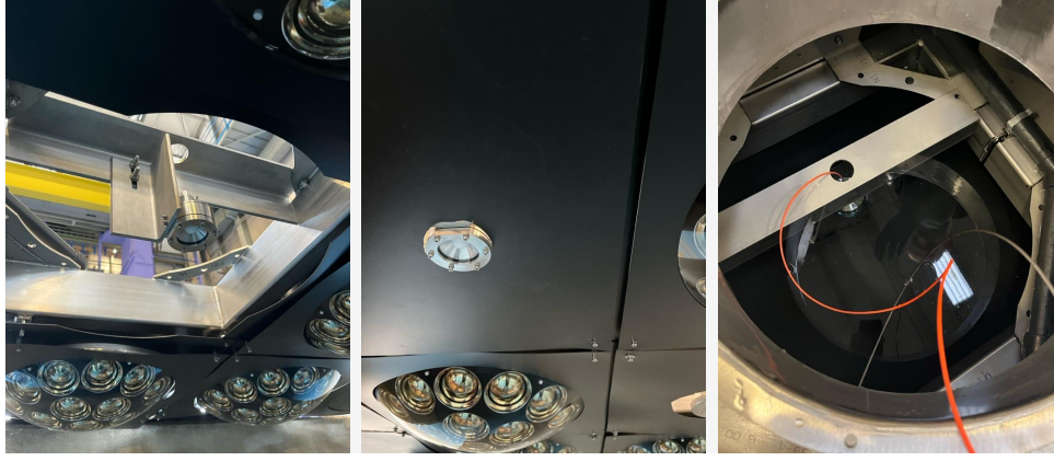
Figure 3.11: Picture of the UKLI diffuser in WCTE (left) during assembly, (centre) after installation of the black sheet and (right) from above the support structure. Picture credit: WCTE collaboration.
