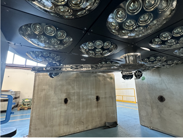
Figure 3.4: Picture of the CDS arm attached to the support structure's top endcap. Picture credit: WCTE collaboration.
