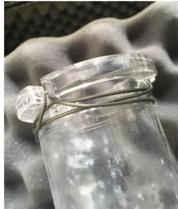
(b) After 4 days of growth, the Kanthal wire broke right at the quartz flange, causing the crucible to fall onto the floor.
