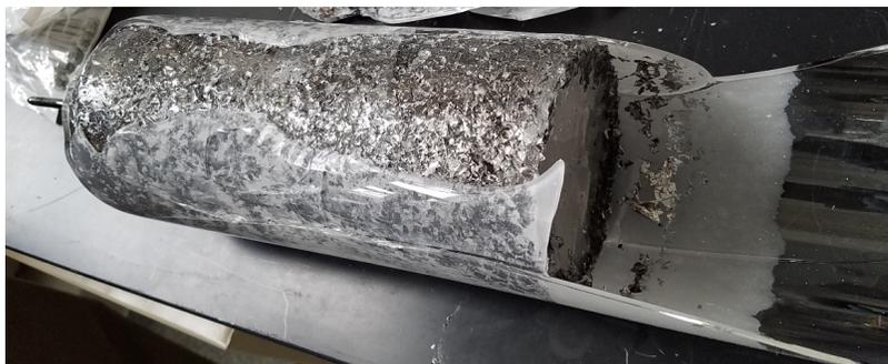
Figure 4.6: NaI-025 failed due to carbon coating peeling off and crucible cracking during cooling. Pieces of pyrolytic carbon is embedded in the crystal. The coating on the top part of the crucible (the right end in picture) is completely consumed due to reaction with oxygen in the air at the elevated temperature after the crucible cracked open. Photo courtesy of RMD.
