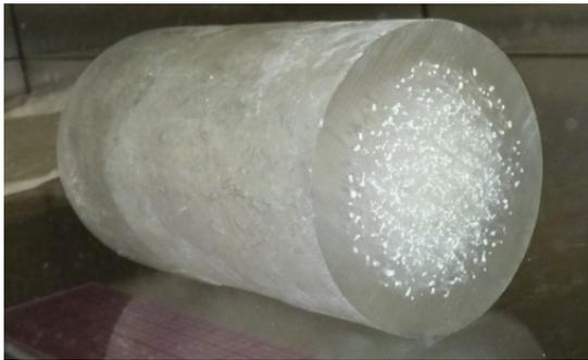
(a) Photo of NaI-026 cross section. NaI-026 had many small bubble-like cavities in the bulk of the crystal. Photo courtesy of RMD.
