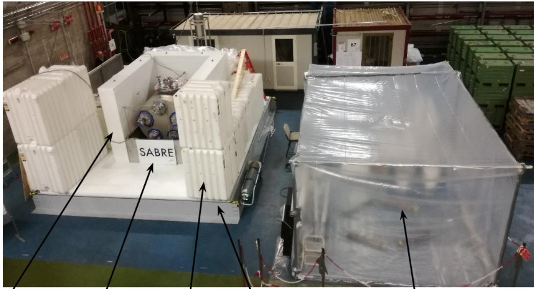
Polyethylene Veto vessel Water Lead Temporary cleanroom
