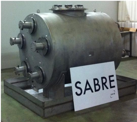
(a) The liquid scintillator veto vessel in LNGS Hall B.
