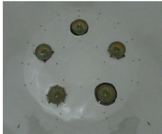
(b) Lumirror lining to improve scintillation light collection efficiency.
