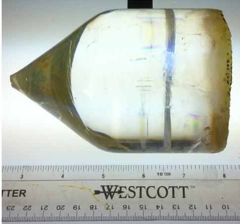
(a) Photo of NaI-014. The crack is not visible from this angle due to total internal refraction of NaI crystal.
