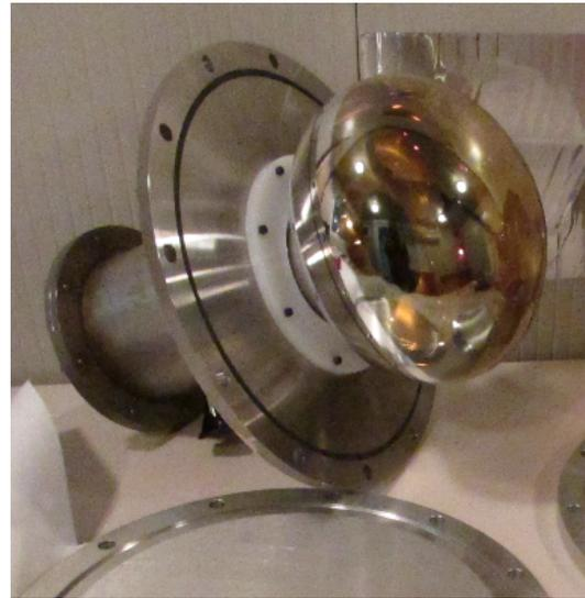
(b) Photo of 8" R5912 PMT mounted onto the PMT holder and PMT can.
