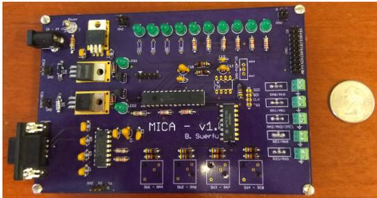
(a) Photo of Mica v0. It uses RS-232 cables to communicate with a PC's serial port.
