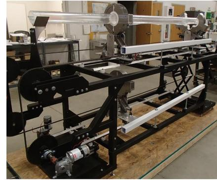
(b) New zone refiner during test.
