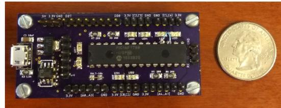
(b) Photo of Lyra v0. Communication to the PC is done using a USB cable and an on-board USB-to-serial converter chip.
