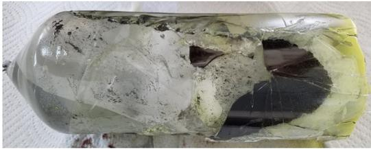
(a) Photo of NaI-032. The carbon coating detached from the crucible and the crystal stuck firmly to the crucible, causing the crucible to eventually break. The yellow color on the right end is due to TII being purified out as crystal grows.
