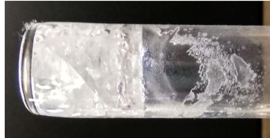
(b) Crystal-grade NaI powder without  $\text{SiCl}_4$  treatment adheres strongly to fused quartz upon crystallization. The quartz is also etched by NaI/NaOH vapor.
