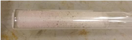
(a)  $\text{SiCl}_4$ -treated Crystal-grade NaI powder crystallized in an uncoated quartz crucible without sticking. The crystal is a polycrystal due to rapid cooling. Compared to the control group, the quartz surface is also cleaner. The gap at the left end is created by sliding the crystal inside the crucible.
