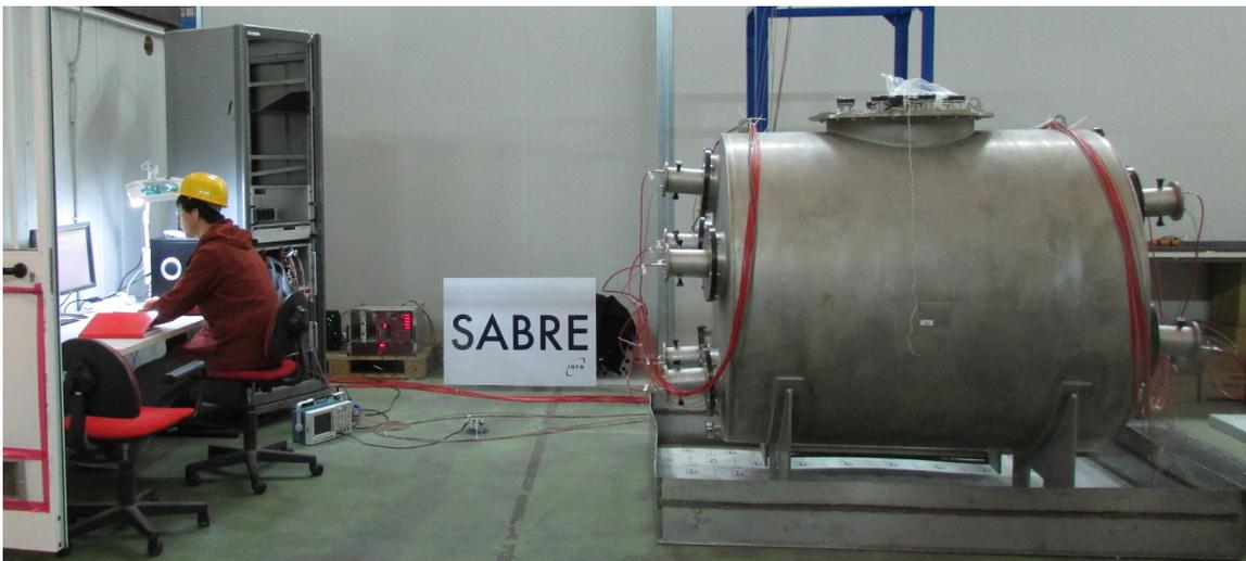
Figure 6.8: Veto detector commissioning at LNGS Hall B. The veto vessel is on the right and the author and the electronics are on the left.
