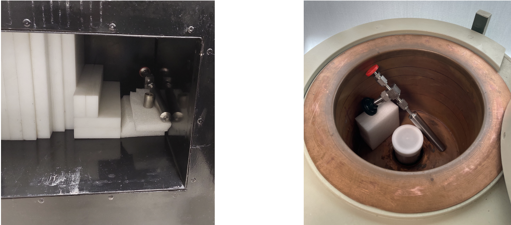
Figure 1. Left: the nano-CaO powder container next to the Am-Be source inside a PE shielding. Right: after irradiation, the container inside the HPGe detector to examine the associated ^{42}\text{K} production.
