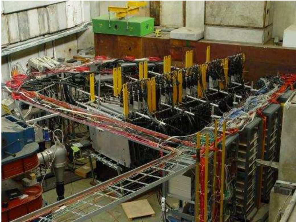
Figure 2.12: A picture of the Calibration Detector in the T7 beamline, assembled at the CERN PS building.
