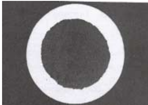
Figure 2-10. Cross-section of monofilamentary BSCCO 2212 wire.
