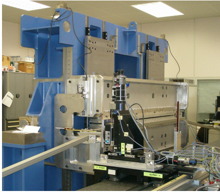
Figure 2: U48 at hall probe measurement bench.
