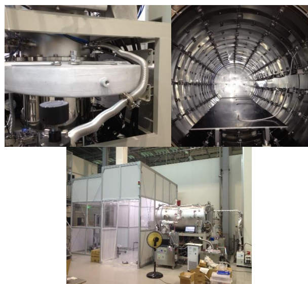
Figure 2: (top left) Water-cooled baffle, gate-valve and cryopump. (top right) Inside furnace. (bottom) Completed furnace with clean booth.
