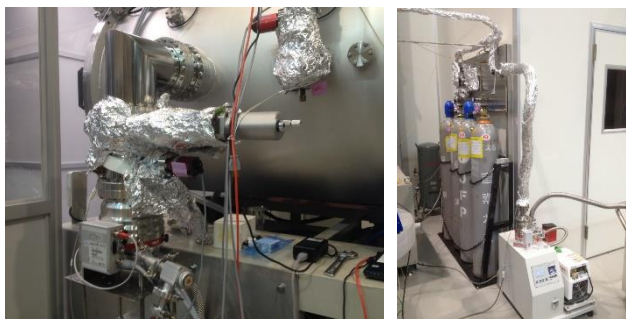
Figure 5: (left) TMP used during Nitrogen-injection. (right) Nitrogen-injection system.
