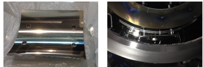
Figure 6: (left) Additional 3 layers of SUS plates. (right) Installed SUS plates between reflectors and a cryopump port.
