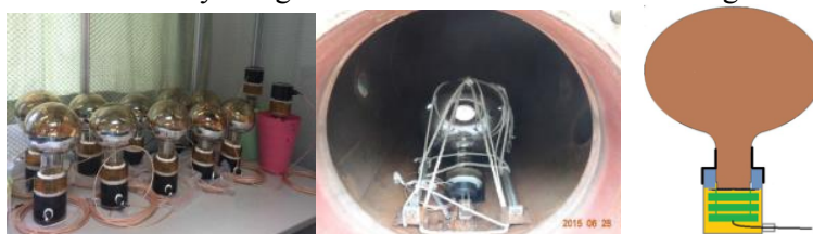
Figure 4. PMT potting: left, 1 st stage potted tubes, middle, pressure test tank, right, latest designed structure for potting with electronics.
