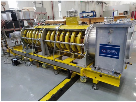
Figure 2: The 648 MHz klystron of CSNS-II Linac superconducting ellipsoidal cavity.
