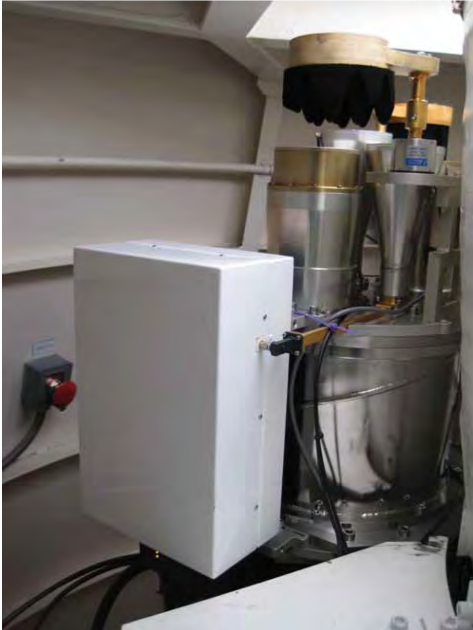
Figure 5.4.15: A side view of the millimetre package with the WVR mounted on the side (the white box). The WVR paddle, feed horn as well as waveguide can be clearly seen. The WVR paddle is in the same position as in Figure 5.4.14, i.e. not obstructing any of the feed horns. Photo by Peter Mirtschin in April 2011.
