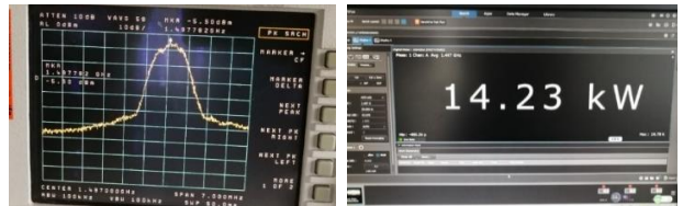
Figure 10: Testing results of 1.5 GHz CW magnetron.
