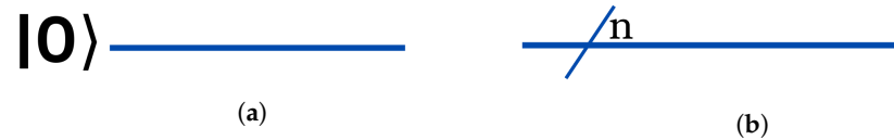
Figure 1. Representations of wires of quantum circuit. (a) Single quantum circuit wire; (b) Quantum circuit wire with n qubits.
