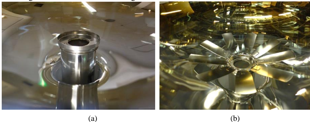
Fig.6. The structure of focusing electrode of different 20-inch MCP-PMT
