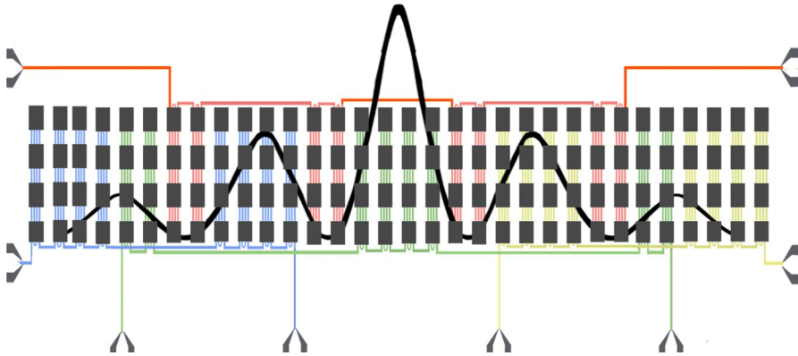
Fig. 6 (Color figure online) Illustration showing one manner in which the rows of detectors could be fed, with 2048 pixels per feedline
