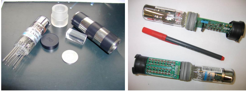
Figure 3.14: Hamamatsu R7899-20 phototube together with the light mixer, mixer housing and permalloy magnetic screen (left) and the Cockcroft-Walton multiplier soldered to the PM (right)
