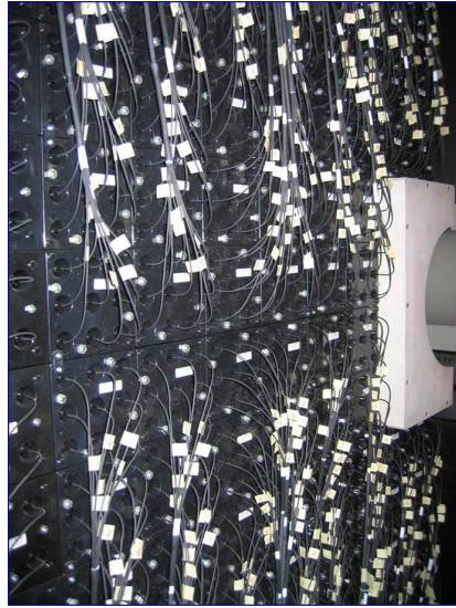
Figure 3.50: Distribution of monitoring signals from LED to the ECAL cells
