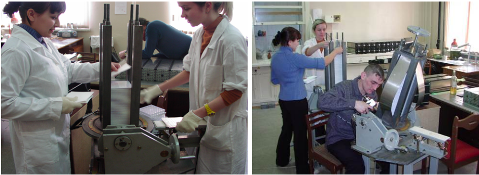
Figure 3.34: Assembly of the outer section module, first stage. Lead-scintillator stack during assembly (left) and pressing the stack and preparing steel tapes for welding (right) are shown
