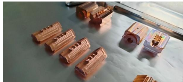
Figure 4: 4-quadrant structure samples before assembly and TIG welding.
