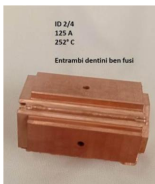
Figure 6: A picture of the cavity taken after the cleaning process to remove the external dirt on the outer surfaces due to the welding.
