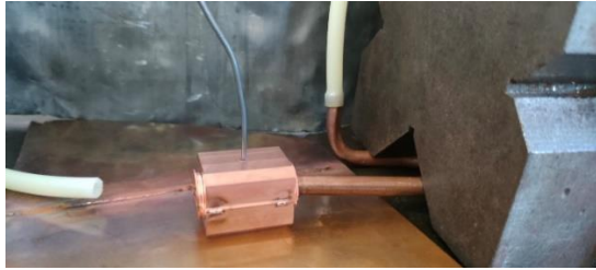
Figure 5: Experimental Set-up for TIG welding. Argon mixture is fused through cavity during welding.
